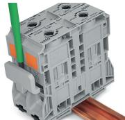
Commoning with an adjacent jumper: insert the jumper above the conductor entry hole – prior to conductor termination. The nominal cross-section remains unchanged.
