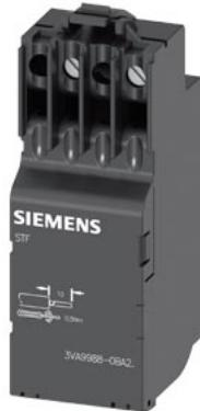
SHUNT TRIP FLEXIBLE 208-277 V AC 50/60 HZ ACCESSORY FOR 3VA10 up to 3VA14 and 3VA20 up to 3VA24
