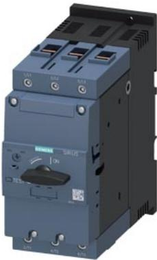
Circuit breaker size S3 for motor protection, CLASS 10 A-release 80...100 A N-release 1300 A screw terminal Standard switching capacity
