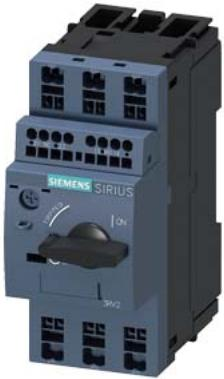
Circuit breaker size S00 for motor protection, CLASS 10 A-release 3.5...5 A N release 65 A Spring-type terminal Standard switching capacity with transverse auxiliary switches 1 NO+1 NC
