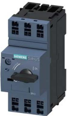
Circuit breaker size S00 for motor protection, CLASS 10 A-release 10...16 A N-release 208 A Spring-type terminal Standard switching capacity
