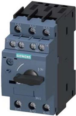
Circuit breaker size S0 for motor protection, CLASS 10 A-release 4.5...6.3 A N-release 82 A screw terminal Standard switching capacity with transverse auxiliary switches 1 NO+1 NC
