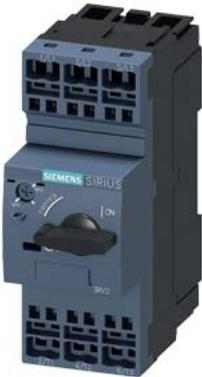
Circuit breaker size S0 for motor protection, CLASS 10 A-release 16...22 A N-release 286 A Spring-type terminal Standard switching capacity
