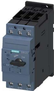
Circuit breaker size S2 for motor protection, CLASS 10 A-release 18...25 A N-release 325 A Screw terminal Standard switching capacity
