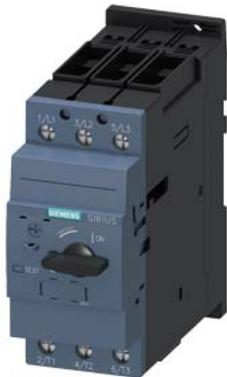
Circuit breaker size S2 for motor protection, CLASS 10 A-release 14...20 A
