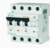
**RCD/MCB combination, 16 A, 30 mA, MCB trip characteristic: C, 3p+N,
