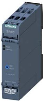
Thermistor motor protection relay Standard evaluation unit 22.5 mm enclosure screw terminal 2 change-over contacts US = 24 V-240 V AC/DC Manual/Auto/Remote reset with ATEX approval 2 LEDs (READY/TRIPPED) Safe galvanic isolation Test/reset button Wire break monitoring Short circuit monitoring non-volatile
