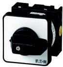
**Spring-return switch, T0, 20 A, flush mounting, 2 contact unit(s), Contacts: 4, Spring-return in START position, 45 °, momentary/maintained, START>1-0-2<START, Design number 8177**
