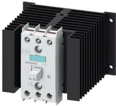
Solid-state contactor 3-phase 3RF2 AC 51 / 40 A / 40 °C 48-600 V / 230 V AC 3-phase controlled screw terminal Blocking voltage 1200 V
