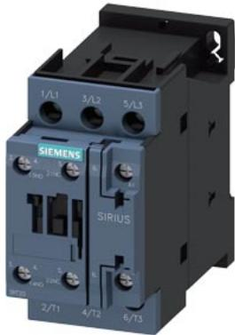
power contactor, AC-3e/AC-3, 9 A, 4 kW / 400 V, 3-pole, 24 V AC, 50 Hz, auxiliary contacts: 1 NO + 1 NC, screw terminal, size: S0
