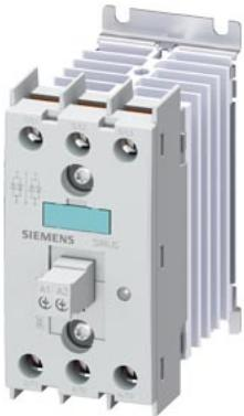
Solid-state contactor 3-phase 3RF2 AC 51 / 10 A / 40 °C 48-600 V / 4-30 V DC 2-phase controlled screw terminal Blocking voltage 1200 V
