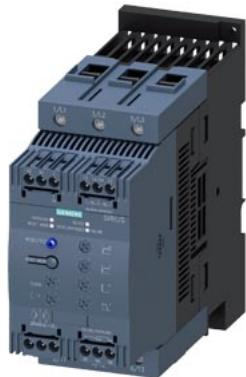
SIRIUS soft starter S3 80 A, 45 kW/400 V, 40 °C 200-480 V AC, 110-230 V AC/DC Screw terminals
