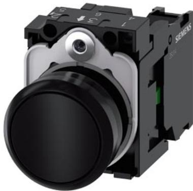
Pushbutton, 22 mm, round, plastic, black, pushbutton, flat, momentary contact type, with holder, 1 NO, screw terminal
