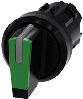
Selector switch, illuminable, 22 mm, round, plastic, green, selector switch, short, 3 switch positions I-O-II, latching, actuating angle 2x45°, 10:30h/12h/13:30h
