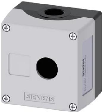
Enclosure for command devices, 22 mm, round, Enclosure material metal, enclosure top part gray, 1 control point, without equipment, Recess for labels, floor mounting, 1xM20 each on top and bottom
