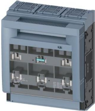
SENTRON, Fuse switch disconnector 3NP1, 3-pole, NH3, 630 A, for assembly and installation on mounting plate, flat terminal, cover level 70 mm
