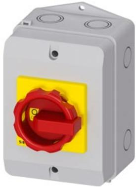
SENTRON, Switch disconnector 3LD, emergency switching-off switch, 3- pole, Iu: 16 A, operating power / at AC-23 A 400 V: 7.5 kW, Molded plastic encapsulation for metric cable gland, rotary operating mechanism, red/yellow
