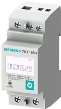
SENTRON, measuring device, 7KT PAC1600, LCD, L-N: 230 V, 63 A, strd rail instr., sing.-ph., Modbus RTU/ASCII + MID, app. /active/reactive energy, self-powered, screw terminals
