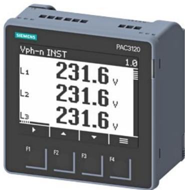
SENTRON PAC3120 LCD 96X96 mm Power Monitoring Device Controll panel instrument for electrical values protocol: Modbus RTU with graphics display U rated input: 690/400V 45-65Hz IE rated input: X/1A oder X/5A AC Power supply: 100 ... 250 V +-10 % AC/DC screw connections
