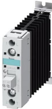
Solid-state contactor 1-phase 3RF2 AC 51 / 30 A / 40 °C 48-460 V / 4-30 V DC short circuit-proof up to 25 A with B miniature circuit breaker
