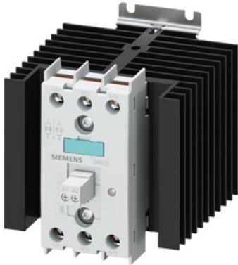
Solid-state contactor 3-phase 3RF2 AC 51 / 40 A / 40 °C 48-600 V / 4-30 V DC 2-phase controlled screw terminal Blocking voltage 1200 V
