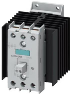
Solid-state contactor 3-phase 3RF2 AC 51 / 20 A / 40 °C 48-600 V / 4-30 V DC 3-phase controlled screw terminal Blocking voltage 1200 V
