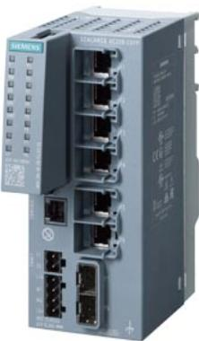
SCALANCE XC206-2SFP manageable Layer 2 IE switch; IEC 62443-4-2 certified; 6x 10/100 Mbit/s RJ45 ports; 2x 100/1000 Mbit/s SFP; 1x console port; diagnostics LED; redundant power supply; temperature range -40 °C to +70 °C; assembly: DIN rail/S7 mounting rail/wall Office redundancy functions features (RSTP, VLAN,...); PROFINET IO device; Ethernet/IP-compliant; C-plug slot;
