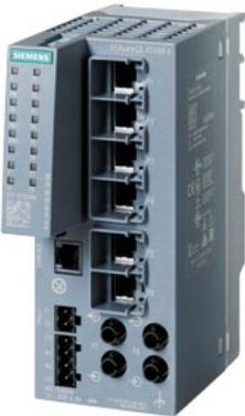
SCALANCE XC206-2 manageable Layer 2 IE switch; IEC 62443-4-2 certified; 6x 100 Mbit/s RJ45 ports; 2x 100 Mbit/s ST/BFOC ports; 1x console port; diagnostics LED; redundant power supply; temperature range -40 °C to +70 °C; assembly: DIN rail/S7 mounting rail/wall redundancy functions; office features (RSTP, VLAN,...); PROFINET IO device; Ethernet/IP-compliant C-PLUG slot;
