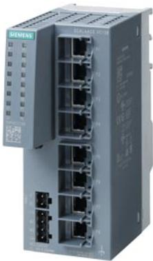
SCALANCE XC108, Unmanaged IE switch, 8x 10/100 Mbit/s RJ45 ports, LED diagnostics, error-signaling contact with set pushbutton, redundant power supply Manual available as a download .
