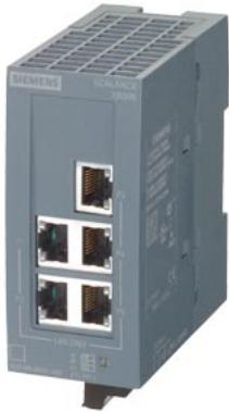
SCALANCE XB005 unmanaged Industrial Ethernet Switch for 10/100 Mbit/s; for setting up small star and line topologies; LED diagnostics, IP20, 24 V AC/DC power supply, with 5x 10/100 Mbit/s twisted pair ports with RJ45 sockets; Manual available as a download .
