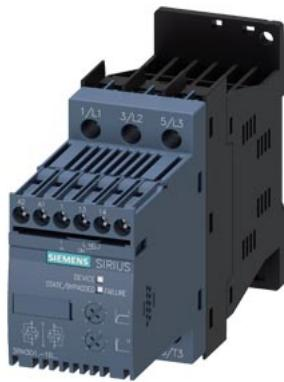
SIRIUS soft starter S00 17.6 A, 7.5 kW/400 V, 40 °C 200-480 V AC, 110-230 V AC/DC Screw terminals
