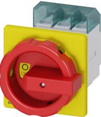
SENTRON, Switch disconnector 3LD, emergency switching-off switch, 3- pole, I<sub>u</sub>: 63 A, operating power / at AC-23 A 400 V: 22 kW, front-mounted, rotary operating mechanism, Red / yellow, central mounting 22.5 mm of the handle
