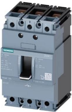
switch disconnector 3VA1 IEC frame 160 3-pole SD100, In=100A without overload protection w/o short-circuit protection nut keeper kit
