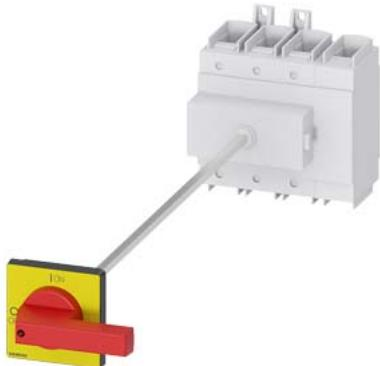
SENTRON, Switch disconnector 3LD, emergency switching-off switch, 4- pole, I<sub>u</sub>=250 A, operating power / at AC-23 A 400 V: 132 kW, floor mounting with door coupling, knob-operated mechanism, red/yellow, 4-hole mounting of the handle
