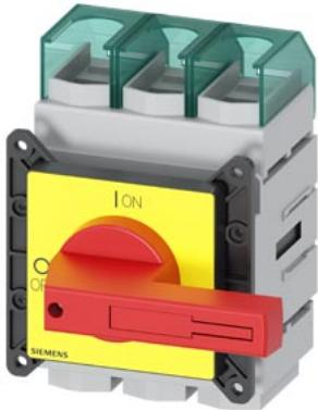
SENTRON, Switch disconnector 3LD, emergency switching-off switch, 3- pole, I<sub>u</sub>=250 A, operating power / at AC-23 A 400 V: 132 kW, front-mounted, knob-operated mechanism, red/yellow, 4-hole mounting of the handle
