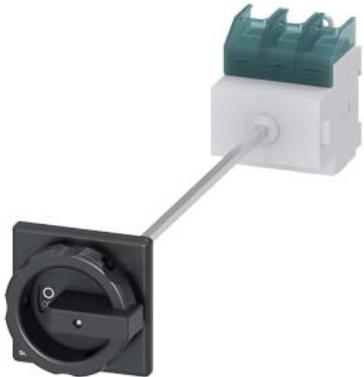
SENTRON, Switch disconnector 3LD, main switch, 3-pole, I<sub>u</sub>: 125 A, Operating power / at AC-23 A at 400 V: 45 kW, floor mounting with door coupling, rotary operating mechanism, black, 4-hole mounting of the handle
