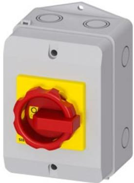
SENTRON, Switch disconnector 3LD, emergency switching-off switch, 3- pole, Iu: 25 A, operating power / at AC-23 A 400 V: 9.5 kW, Molded plastic encapsulation for metric cable gland, rotary operating mechanism, red/yellow
