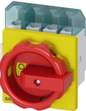
SENTRON, Switch disconnector 3LD, emergency switching-off switch, 4- pole, Iu: 32 A, operating power / at AC-23 A 400 V: 11.5 kW, front-mounted, rotary operating mechanism, Red / yellow, 4-hole mounting of the handle
