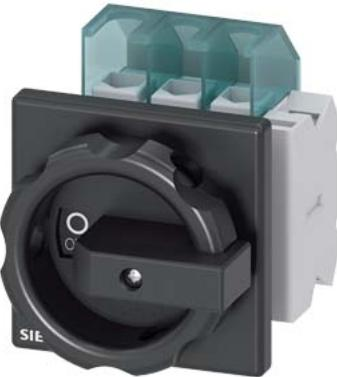
SENTRON, Switch disconnector 3LD, main switch, 3-pole, I<sub>u</sub>: 25 A, Operating power / at AC-23 A at 400 V: 9.5 kW, front-mounted, 1 NC, 1 NO, rotary operating mechanism, black, 4-hole mounting of the handle
