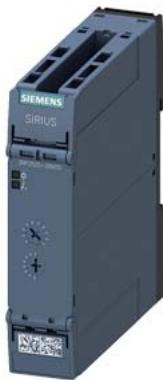
Timing relay, electronic on-delay 2 change-over contacts, 7 time ranges 0.05 s...100 h 12-240 V AC/DC at 50/60 Hz AC with LED, Spring-type terminal (Push-In)
