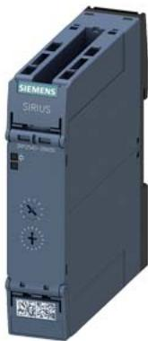
Timing relay, electronic OFF delay without control signal or smooth passing make contact non-volatile 7 time ranges 0.05...600 s 12-240 V AC/DC at 50/60 Hz AC, 2 change-over contacts with LED Spring-type terminal (push-in)
