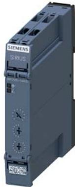
Timing relay, Multifunction 1 change-over contact, 13 functions 7 time ranges (0.05 s...100 h) 12...240 V AC/DC at 50/60 Hz AC with LED, Screw terminal
