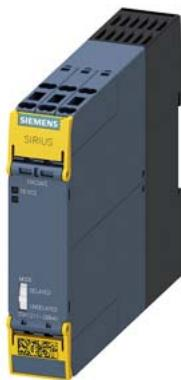
SIRIUS safety relay Output expansion 4RO with relay enabling circuits 4 NO contacts plus Relay signaling circuit 1 NC contact Us = 24 V DC Spring-type terminal (push-in)
