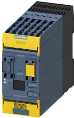
SIRIUS safety relay basic unit 3SK2 series 20 F-DI, 4 F-DQ, 2 DQ, 24 V DC Can be parameterized via SIRIUS Safety ES 45 mm width screw terminal up to SIL 3 (IEC 62061) up to performance level e (ISO 13849-1) output expansions 3SK1, coupling relay 3RQ1 and fail-safe motor starters 3RM1 via device connector connectable
