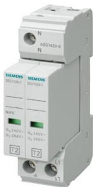
Surge arrester Type 2 Requirement class C, UC 350V Pluggable protective modules 2-pole, 1+1 circuit for TN-S and TT systems Narrow design
