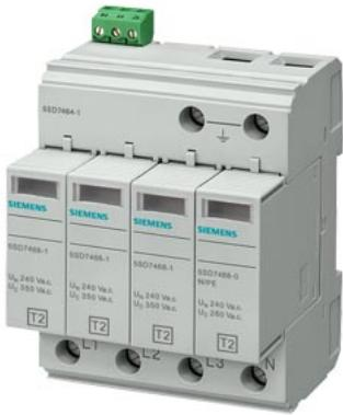
Surge arrester Type 2 Requirement class C, UC 350V Pluggable protective modules 4-pole, 3+1 circuit for TN-S and TT systems with remote display
