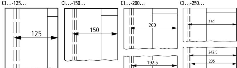
Mounting depth with mounting rail 7.5 mm or 15 mm
