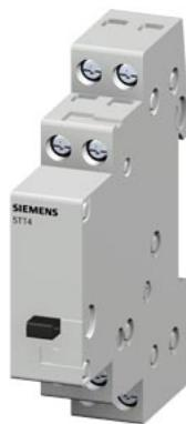
Remote control switch with 1 NO contact, and 1 NC Contact for 230 V AC, 400V 16A Control 24 V DC
