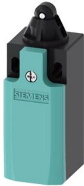
Position switch Plastic enclosure according to EN 50047, 31 mm Device connection 1 x (M20 x 1.5) 1 NO/1 NC quick action contacts integrated (not replaceable) Roller plunger, Form C with plastic roller 10 mm
