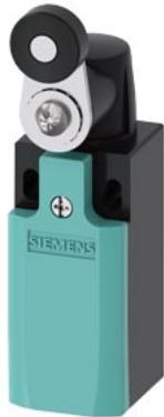
Position switch Plastic enclosure according to EN 50047, 31 mm Device connection 1 x (M20 x 1.5) 1 NO/1 NC quick action contacts integrated (not replaceable) Twist lever, 21 mm long right/left adjustable with plastic roller 19 mm
